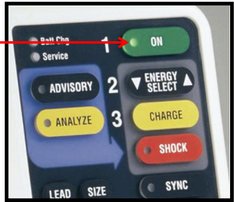
“ON” button does not shock
